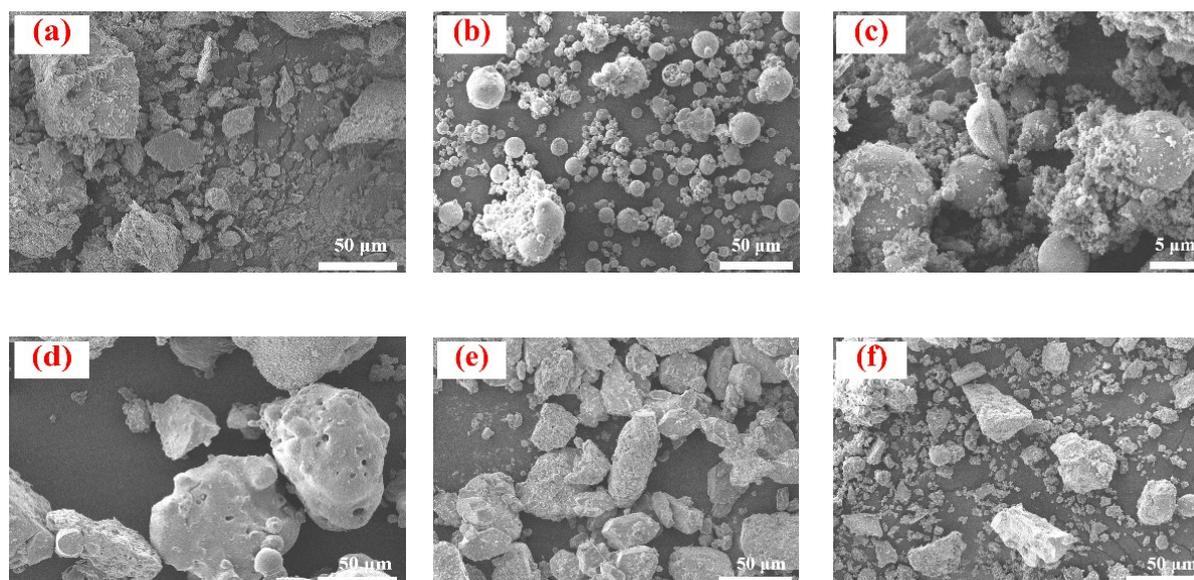
**Figure 5.** SEM microstructure of coal-based solid waste filling material, with (a) coal gangue, (b) fly ash, (c) gasification slag, (d) furnace bottom slag, (e) desulfurization gypsum, and (f) cement in the figure.
