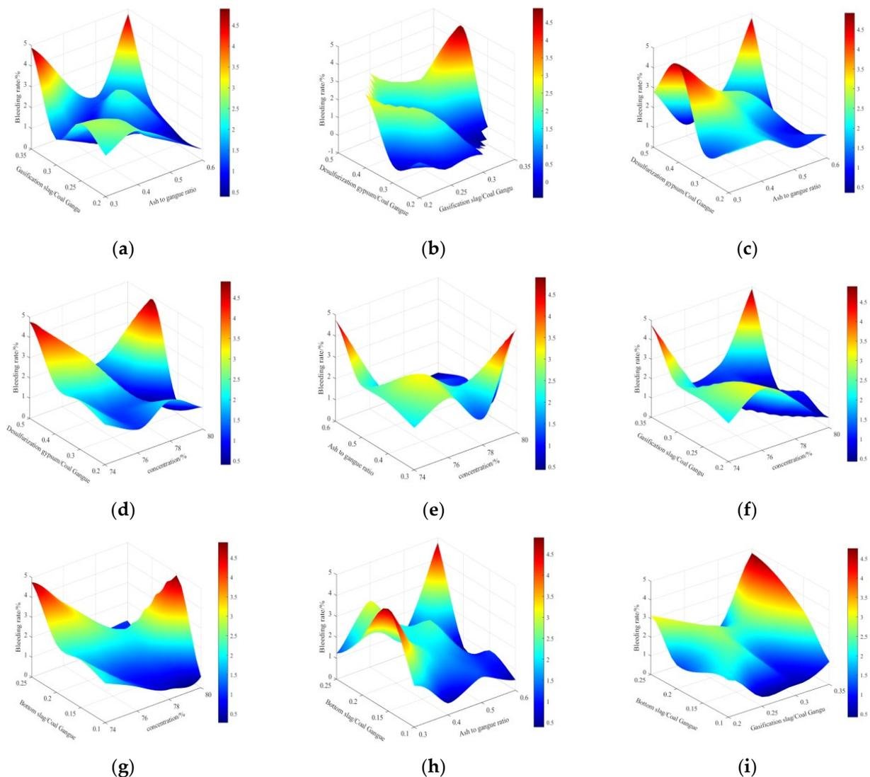
**Figure 12.** Effect of coal-based solid waste filling material on bleeding rate. (a) Factors of B and C; (b) factors of C and E; (c) factors of B and E; (d) factors of A and E; (e) factors of A and B; (f) factors of A and C; (g) factors of A and D; (h) factors of B and D; (i) factors of C and D.
