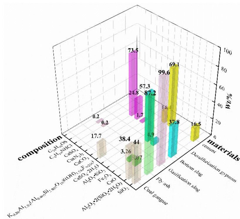
Figure 3. Analysis of main components of coal-based solid waste filling materials.
