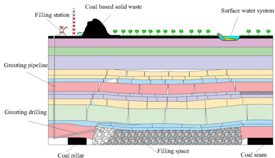
**Figure 2.** Application of coal-based solid waste in paste filling.
