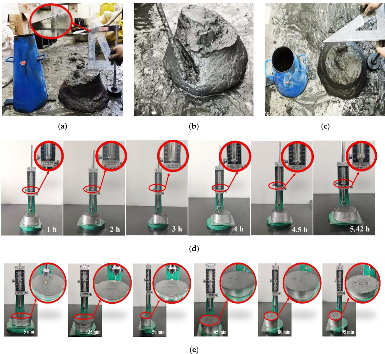
**Figure 14.** Engineering performance inspection of coal-based solid waste filling body. (a) Slump test; (b) cohesion test; (c) water retention test; (d) initial setting time test; (e) final setting time test.
