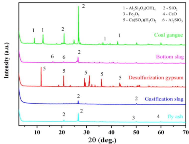
Figure 4. X-ray diffraction (XRD) of coal-based solid waste filling material.
