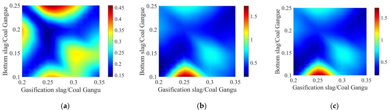
**Figure 13.** Influence of C and D factors on compressive strength of different curing ages. (a) 3 d UCS; (b) 7 d UCS; (c) 28 d UCS.
