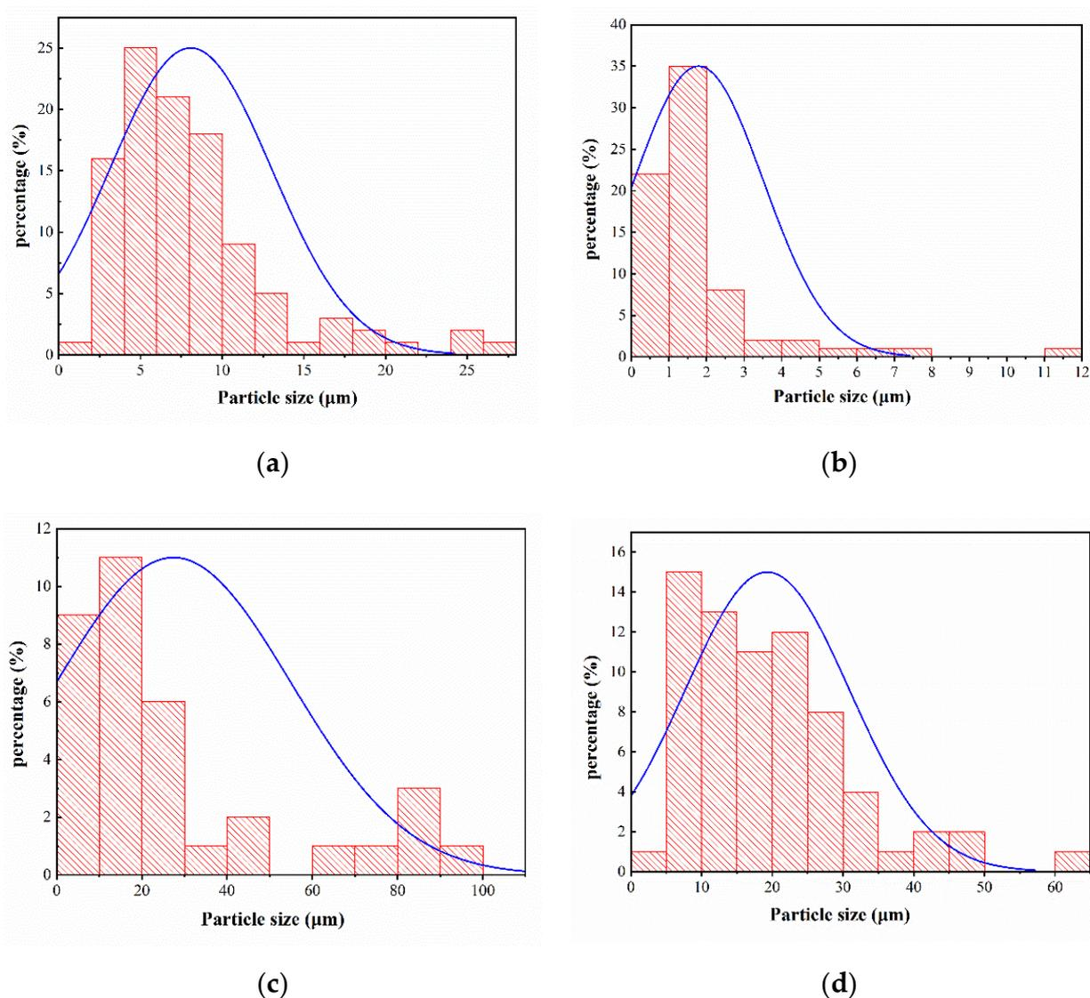
**Figure 7.** Particle size distribution diagram of coal-based solid waste materials, including (a) fly ash, (b) gasification slag, (c) bottom slag, (d) desulfurized gypsum.
