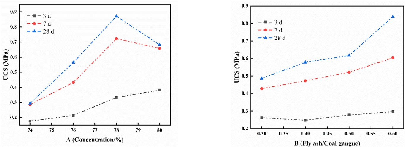
Figure 10. Influence of concentration and ash/gangue ratio on strength development.
