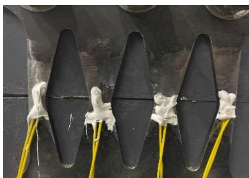
**Figure 6.** Energy dissipator with strain gauges.
