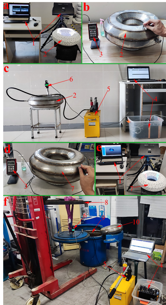
Figure 12. Experimental flowchart of toroidal pressure hull: (a) surface scanning of preformed toroid, (b) thickness measuring of preformed toroid, (c) internal hydroforming of preformed toroid, (d) thickness measuring of hydroformed toroid, (e) surface scanning of hydroformed toroid, and (f) hydrostatic testing of hydroformed toroid.
