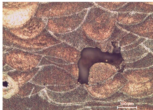
Figure 16. Porosity in a longitudinal section.
