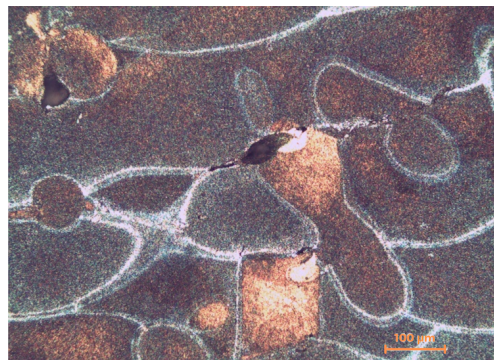
Figure 15. Porosity in a transversal section.
