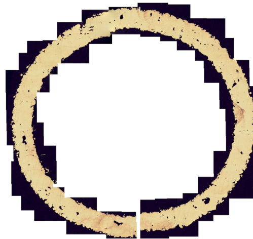
Figure 13. Porosity in a 1.2 specimen transversal section due to low energy density.
