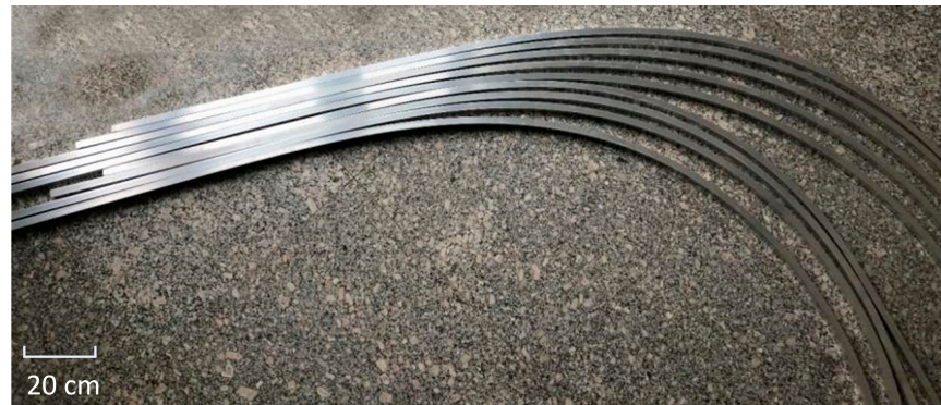
Figure 12. Partially variable-curvature experimental profiles.
