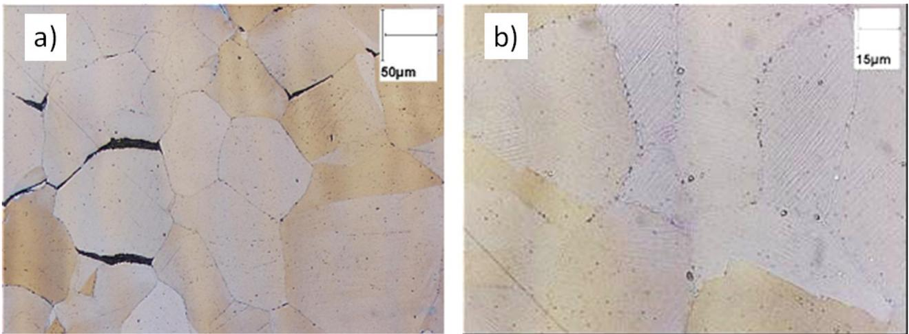
Figure 9. Optical micrographs of solution-treated 0.2 wt.% V steel after testing at 800 °C at a section close to the point of failure (a) showing intergranular cracking (200×) and (b) the presence of precipitates decorating the austenite grain boundaries (500×).
