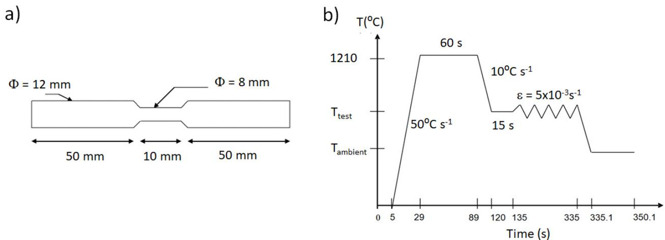
**Figure 2.** Schematic diagrams showing (a) the tensile test specimen geometry and (b) the thermomechanical testing cycle.
