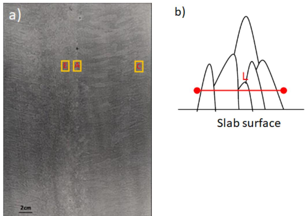
**Figure 3.** (a) Macroscopic etch of a continuous cast slab of steel 6A (containing 0.2 wt.% V and 0.032 wt.% P) showing the solidification structure and the positions of the columnar grain (C), equiaxed grain (E) and axial (A) regions chosen for EPMA, (b) illustration of the method used for austenite grain size measurement.
