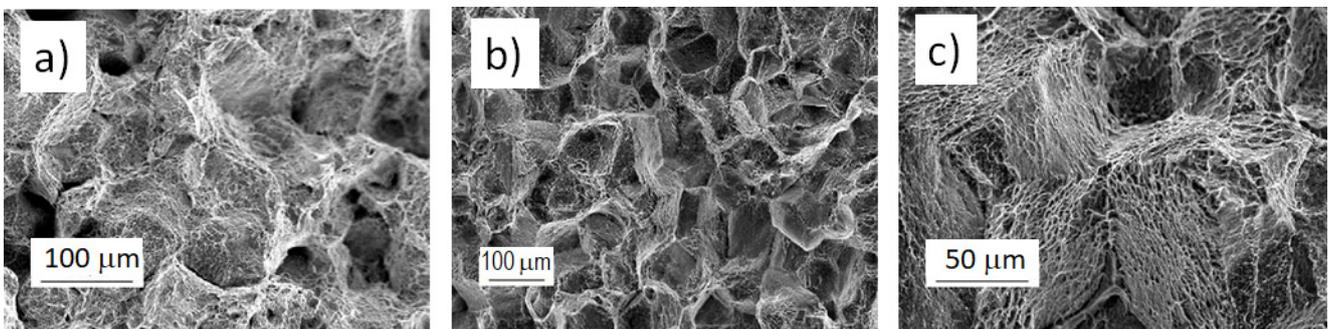
Figure 10. (a) Steel 3A (V-free) solution-treated and strained at 800 °C, (b,c) Steel 5A (0.21 wt.% V) solution-treated and strained at 762 °C.
