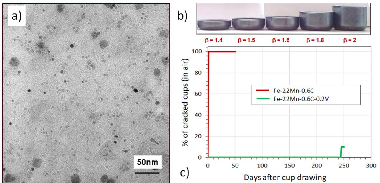
**Figure 1.** (a) TEM replica of V(C,N) in cold-rolled Fe-0.6C-22Mn-0.2V-0.01N; (b) deep-drawn cups used for HE testing; and (c) the effect on crack formation in fully drawn cups [17].
