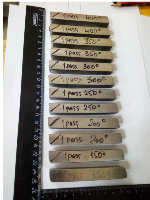
Figure A2. The steel AISI 321L workpieces after ECAP at different temperatures.
