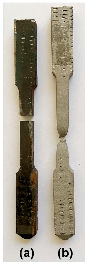
**Figure 4.** Broken tensile specimens: (a) aged specimen; (b) specimen in as-printed state.
