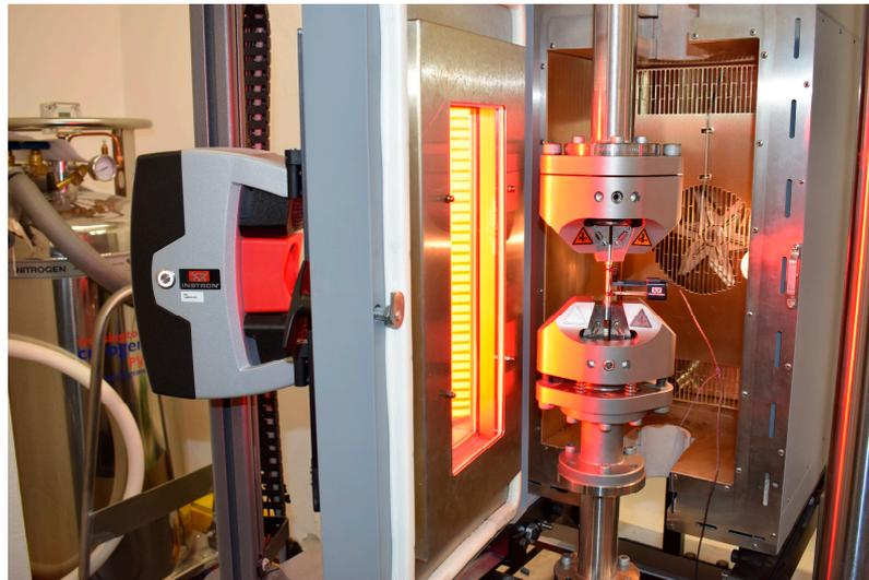
**Figure 3.** Measuring system with a temperature chamber.
