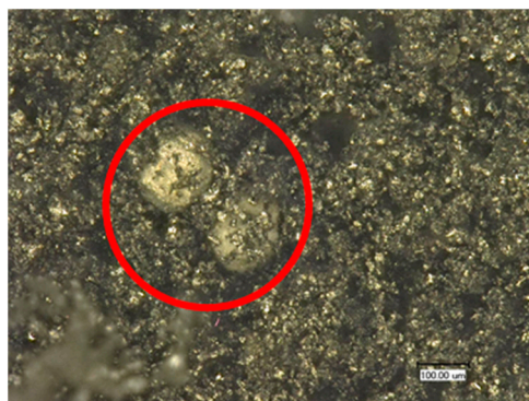
Figure 10. A light microscope image of a <500 μm fraction from the pyrolysis trial at 718 °C with molten particles.
