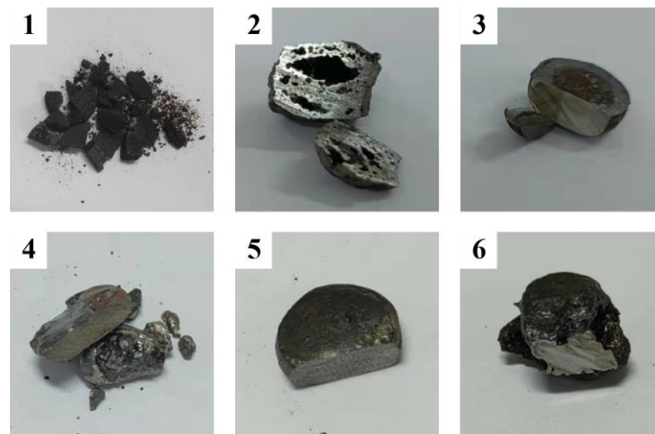
Figure 3. Appearance of the alloy after reduction: (1) 1250 °C, 13% C; (2) 1350 °C, 13% C; (3) 1450 °C, 13% C; (4) 1400 °C, 10% C; (5) 1400 °C, 13% C; (6) 1400 °C, 16% C.
