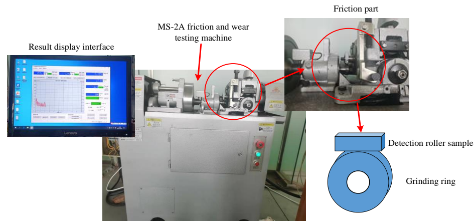
Figure 3. MS-2A friction and wear testing machine.
