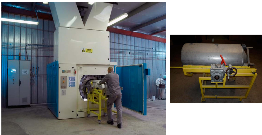
Figure 1. Rotating furnace on left where the sample container is installed as seen on right.
