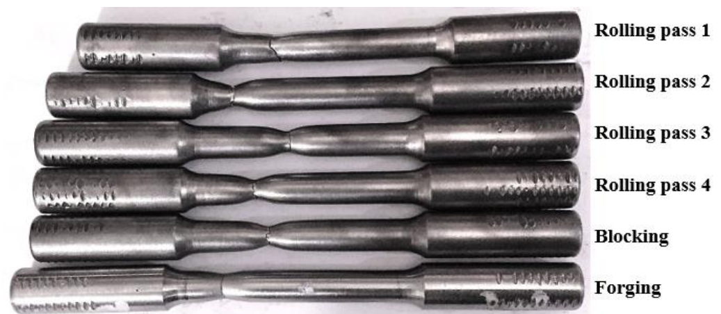
Figure 6. Fractured tensile test specimen after each MSR, blocking and forging stage.
