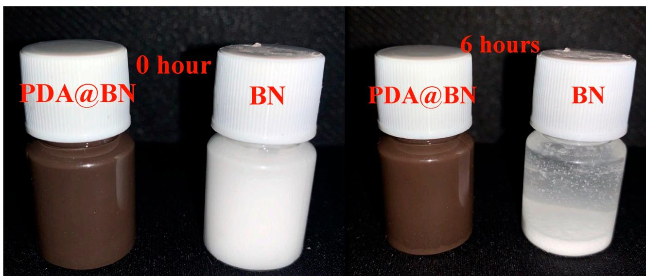
**Figure 2.** The dispersion stability of PDA@BN and BN nanosheets (0.60 g/L) in a phosphating bath at 0 and 6 h was examined visually, as shown in the digital photos.
