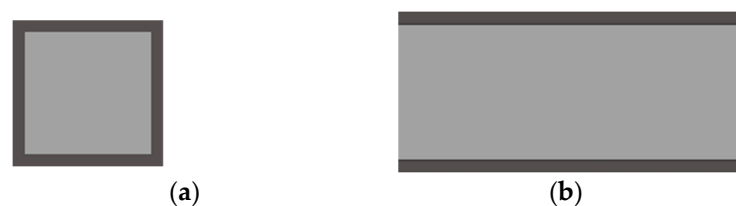
Figure 7. Composite material model (CMM) of the oxidized creep sample. A soft interior zone (pure Ti, light grey) is surrounded by an external hard zone (oxygen-rich Ti, dark grey) of depth x_H . (a) section, side 3 mm; (b) gauge length (tensile axis is horizontal). For the sake of simplicity, the hard zone is homogeneous in oxygen content and properties, an obvious deviation from the real case.
