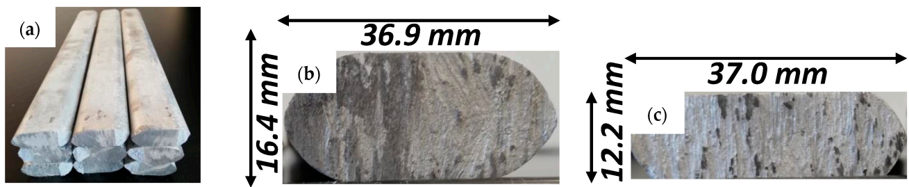
Figure 2. Cross-sectional area of the aluminum alloy sample. (a) Original (As-cast), (b) before the rolling/forging process, and (c) after applying the rolling/forging process.
