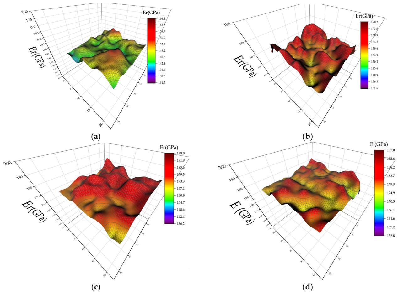
**Figure 12.** Three-dimensional map representation of  $E$ , denoting the difference in nanoindentation response due to phase properties underneath the indenter, for (a) Blend 1 XY, (b) Blend 1 XZ, (c) Blend 2 XY plane, (d) Blend 2 XZ plane.
