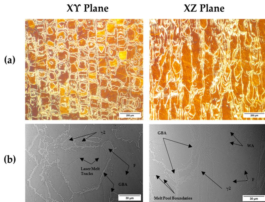
**Figure 7.** Blend 1 as-built microstructure. (a) LOM (Light Optical Microscope) and (b) SEM (Scanning Electron Microscope) micrographs transverse to the build direction (XY plane) and parallel to the build direction (XZ plane). F = Ferrite,  $\gamma_2$  = Secondary Austenite, GBA = Grain Boundary Austenite, WA = Widmanstätten Austenite.
