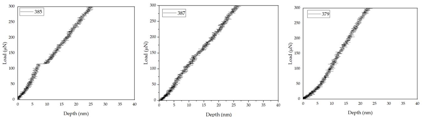
**Figure 13.** Initial part of the loading curve for 3 different points of indentation; the occurrence or lack of pop-ins (or yield type pop-ins) are associated with phase properties underneath the indenter.
