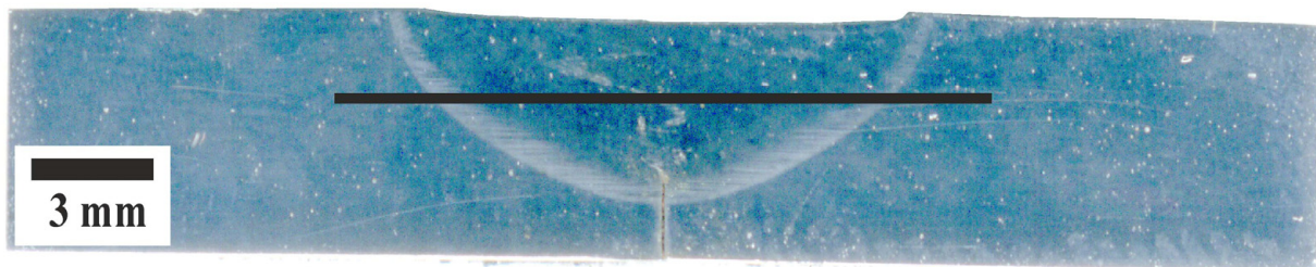
Figure 3. Cross section of the FSW joint sample.
