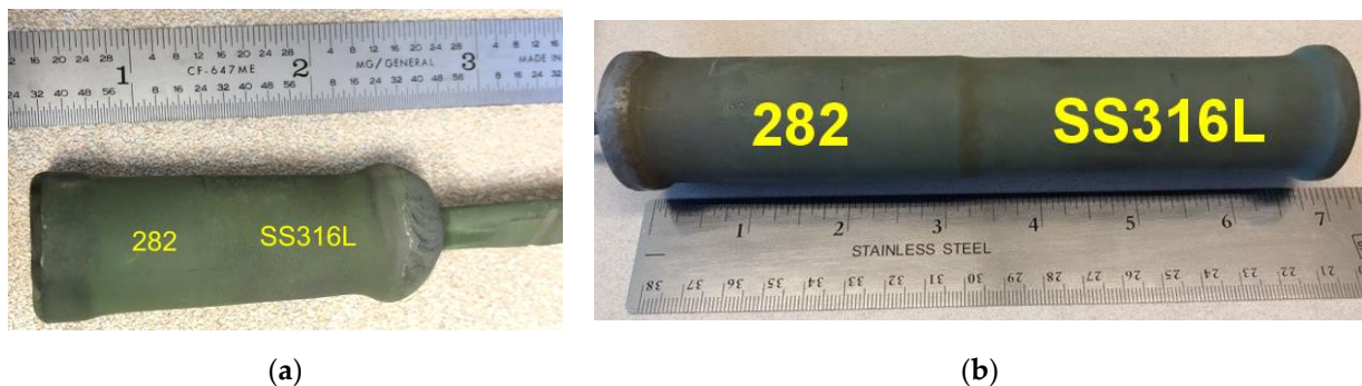
Figure 1. Examples of a small can loaded with SS316L and 282 powder (a) and a taller can loaded with SS316L and 282 powder (b) after HIP cycle.
