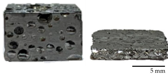
Figure 7. Al foam before and after compression testing.
