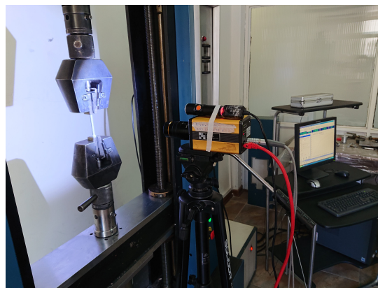
Figure 2. Experimental setup of the tensile tests: an overview of 10-ton Instron universal testing machine, the force register system, and the high-speed camera used for employing digital image correlation.
