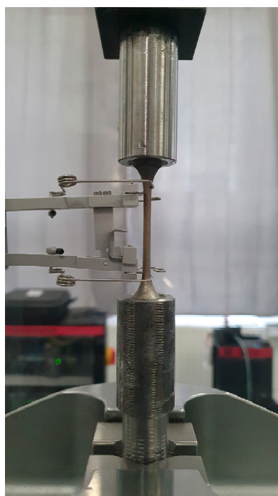
Figure 12. Mounting of the extensometer on a tensile specimen.
