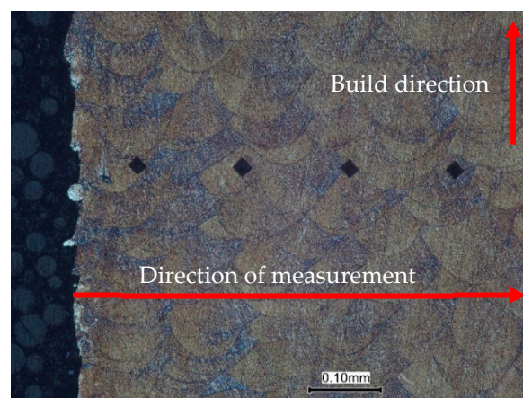
Figure 16. Positions of Vickers hardness measurements.
