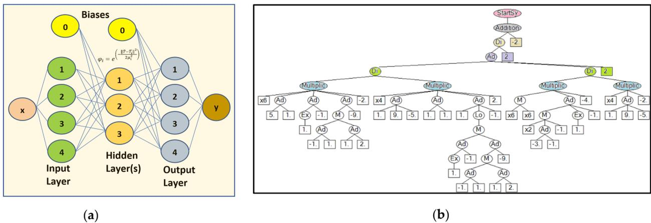
Figure 3. (a) NN architecture for RBF interpolation; (b) tree-like GASR diagram for genetic algorithm fitting.
