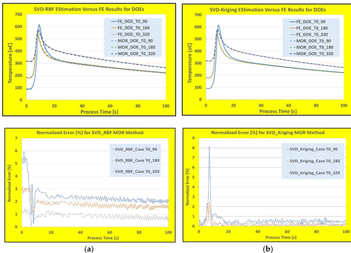
**Figure 5.** Comparison of temperature time histories for FE versus ROMs along with their normalized errors for (a) SVD-RBF trained, and (b) SVD-Kriging ROM techniques.
