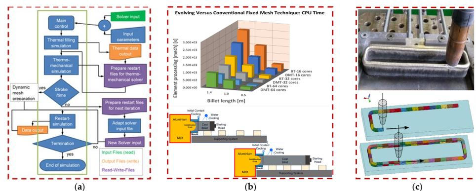
**Figure 1.** (a) Flowchart for evolving algorithm, (b) CPU time comparison for DAT and DMT for horizontal casting case using different numbers of computational cores. Reprinted from Ref. [12], and (c) dynamic WAAM deposition and its numerical mesh-insertion technique for DMT. Reprinted with permission from refs. [16]. 2020, ELSEVIER.
