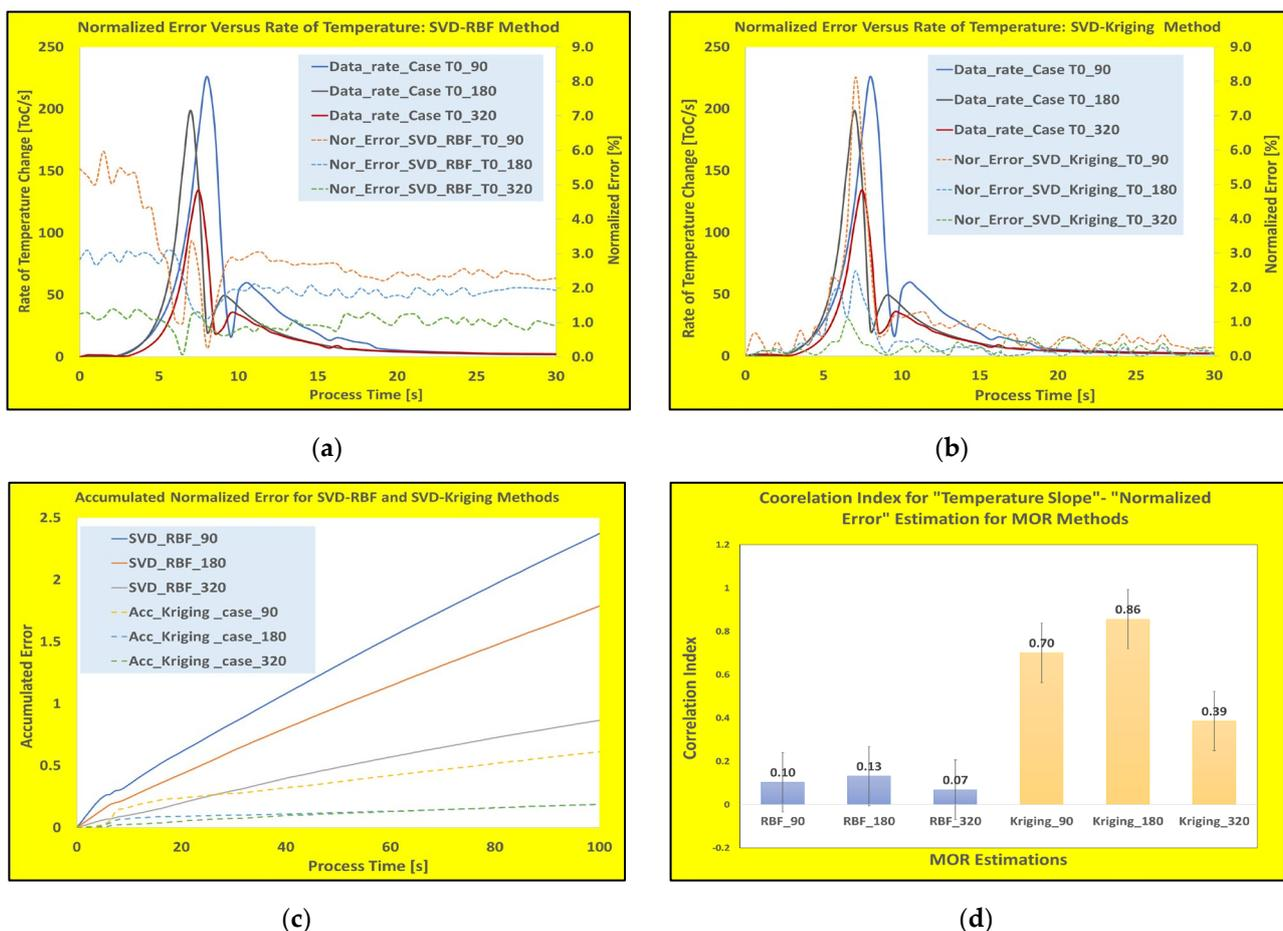
**Figure 6.** Rate of temperature changes (heating rate) versus normalized errors for (a) SVD-RBF trained, (b) SVD-Kriging, (c) accumulated normalized errors for SVD-RBF and SVD-Kriging, and (d) Pearson correlation index for heating rate with respect to normalized error for both techniques.
