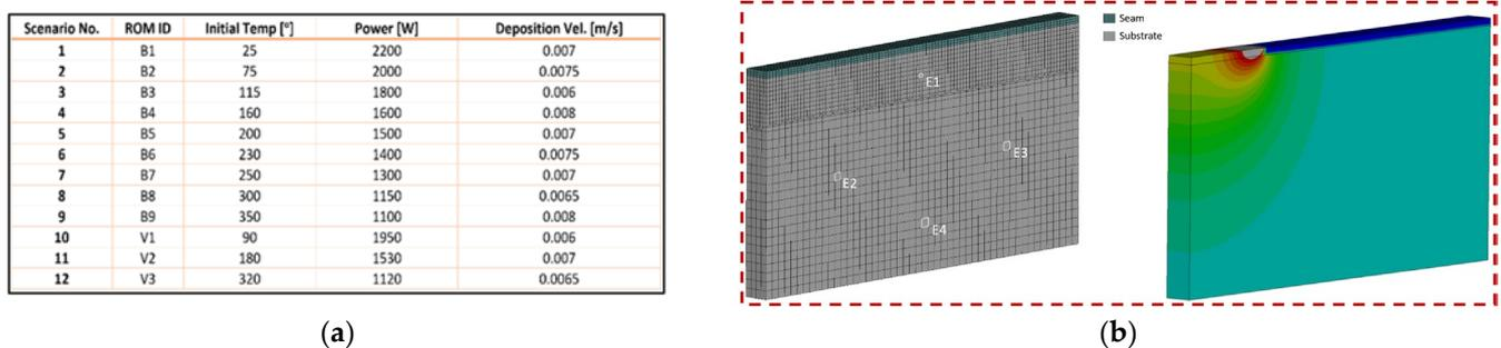
**Figure 2.** (a) Snapshot matrix for WAAM scenarios with varying process parameters; (b) FE mesh with selected measuring points and representative temperature contour during passage of torch. Reprinted with permission from ref. [5].
