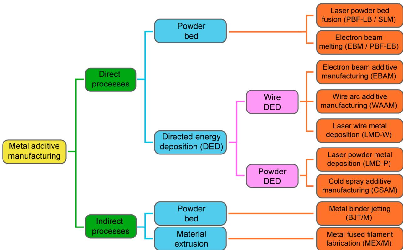
**Figure 1.** Classification of AM techniques for metals.
