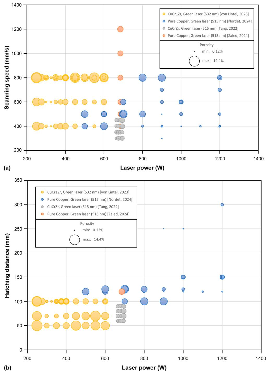
**Figure 7.** Porosity of PBF-LB copper and copper alloy samples reported from Refs. [26,46,54,55], shown as function of process parameters: scanning speed vs. laser power (a); hatching distance vs. laser power (b).
