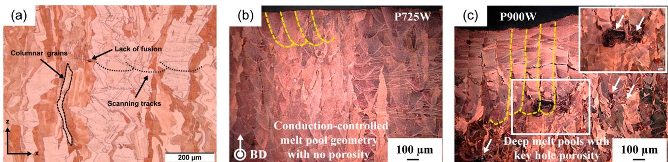
**Figure 10.** Microstructural characterization of pure copper manufactured by: (a) green laser with a linear energy density of 0.81 J/mm. Reprinted from Ref. [20]; (b) IR laser PBF with a linear energy density of 2.25 J/mm. Reprinted from Ref. [45]; (c) IR laser PBF with a linear energy density of 1.82 J/mm. Reprinted from Ref. [45]. Yellow dashed lines indicate melt pools, while white arrows highlight keyhole porosities.
