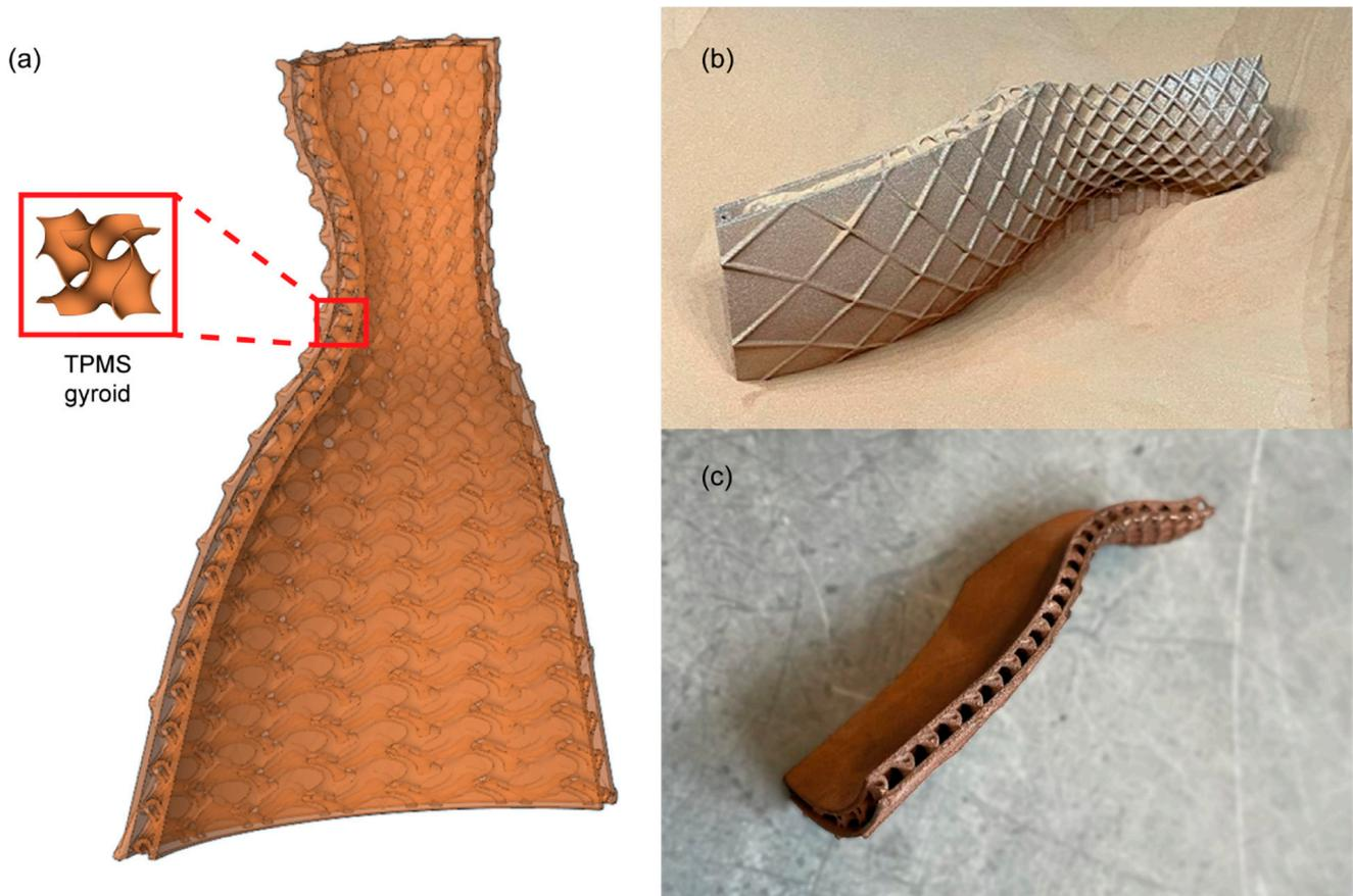
**Figure 18.** Proof of concept for a combustion chamber with self-supporting TPMS structure for cooling: CAD model (a); as-built copper PBF-LB part after powder removal (b); finished part after sand blasting (c).
