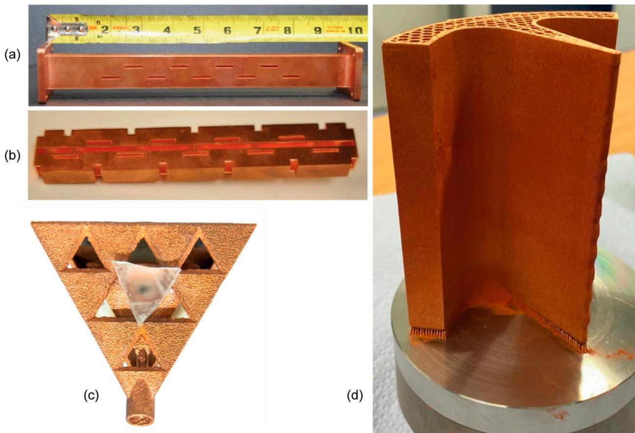
**Figure 17.** Closed (a) and open structure (b) of an X-band slot array waveguide, reprinted from Ref. [97]; RF pyramidal antenna with fractal structure manufactured by green laser PBF (c), reprinted from Ref. [100]; AM radio frequency quadrupole accelerator (d), reprinted from Ref. [101].
