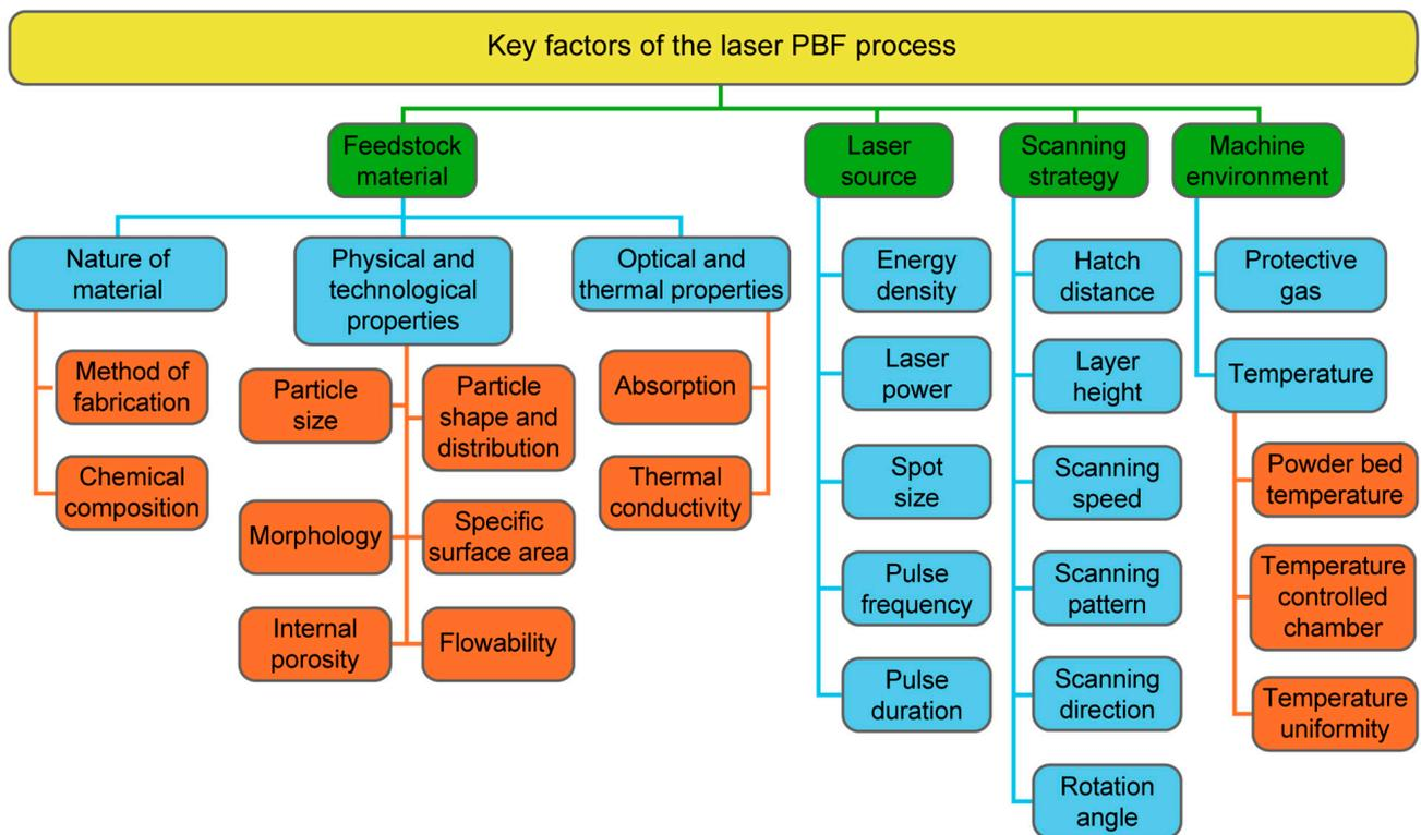
**Figure 6.** Classification of the key factors of the PBF-LB process. Adapted with permission from ref. [27]. 2024 Elsevier.
