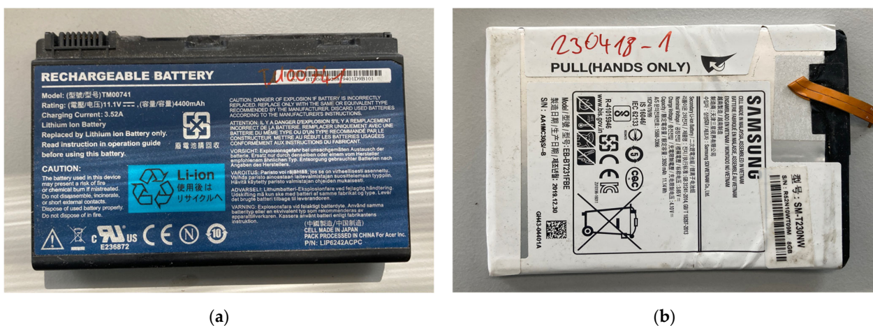
Figure 10. Exemplary LIBs from smartphone, tablet and laptop usage: (a) spent laptop LIB cell type TM00741, Acer Inc. (New Taipei City, China), cylindrical cell, voltage 11.1 V, capacity 4400 mAh; (b) spent tablet LIB cell type SM-T230NW, Samsung (Suwon, Republic of Korea), pouch cell, voltage 3.65 V, capacity 3050 mAh.
