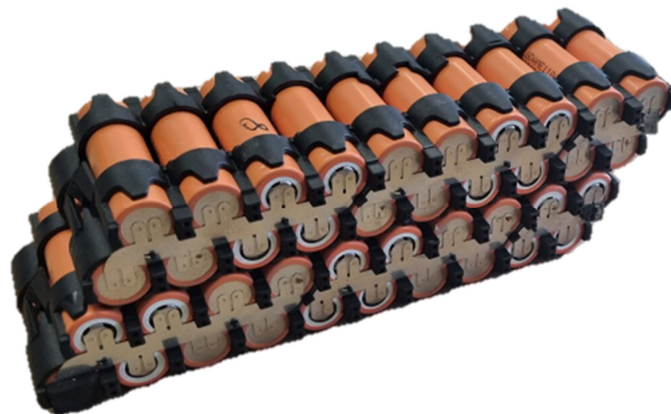
Figure 8. Lithium-ion battery pack Bosch Powerpack Classic 300/400/500—36 V with 500 Wh. Adapted from Ref. [116].
