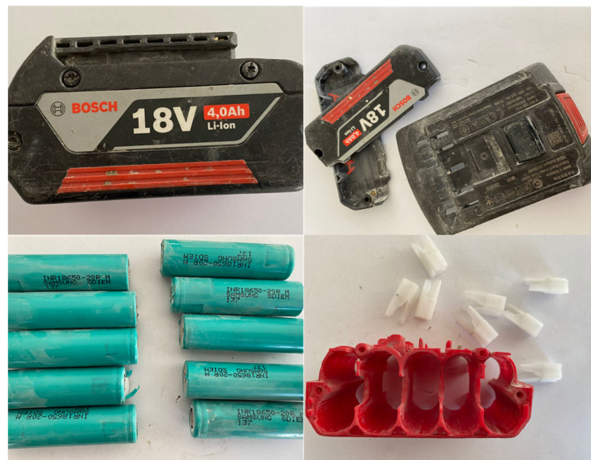
Figure 6. Structure of PT battery pack type TM 51NR19/65-2, voltage 18 V, capacity 4000 mAh, manufacturer: Robert Bosch Powertools GmbH, Leinfelden-Echterdingen, Germany (top left: overall view of the module, top right: dismantled PA66 housing halves, bottom left: cell pack 10 × 3.6 18650 LIB, bottom right: HDPE inner housing).
