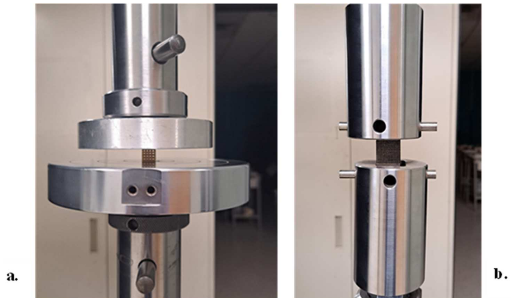
Figure 4. Compression testing setup (a) and tensile testing setup (b). Reprinted from ref. [41].
