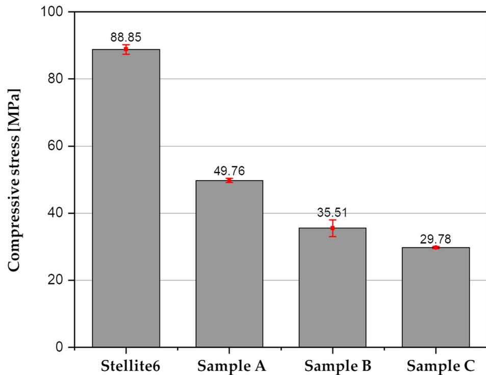
Figure 7. Yield strength changes according to the compression experiment.
