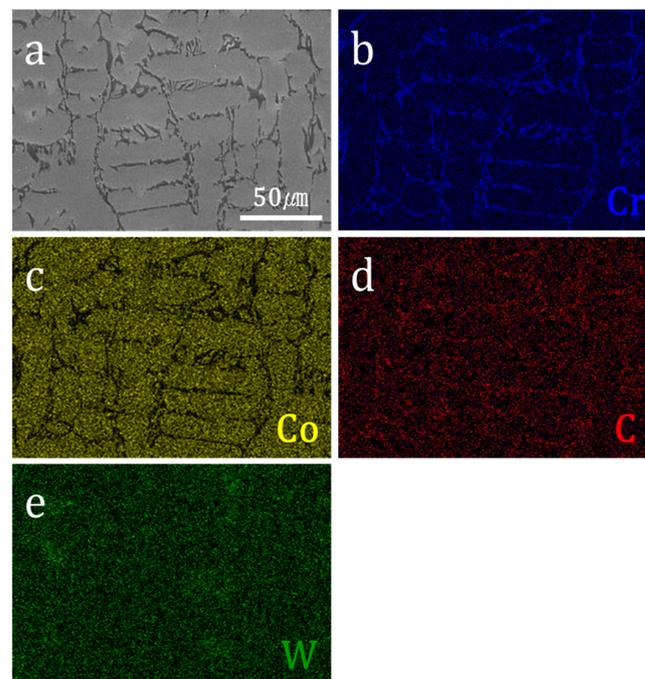
**Figure 3.** EDS mapping image of Stellite 6: (a) SEM image, (b) Cr mapping result, (c) Co mapping result, (d) C mapping result, (e) and W mapping result.
