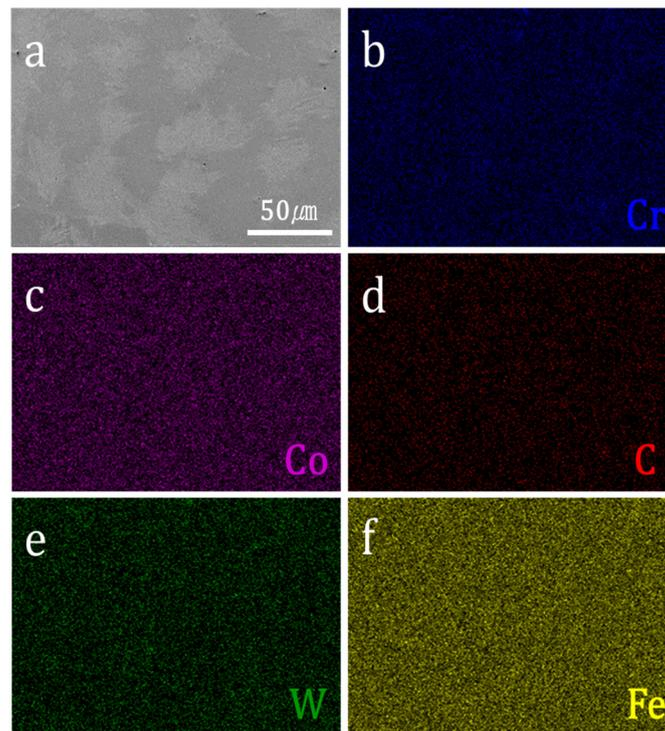
**Figure 4.** EDS mapping image of sample C. (a) Sem image, (b) Cr mapping result, (c) Co mapping result, (d) C mapping result, (e) W mapping result, and (f) Fe mapping result.
