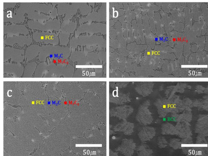
**Figure 2.** BSED image of Stellite according to the amount of Fe added: (a) Stellite 6 image, (b) Sample A image, (c) Sample B image, (d) and Sample C image.
