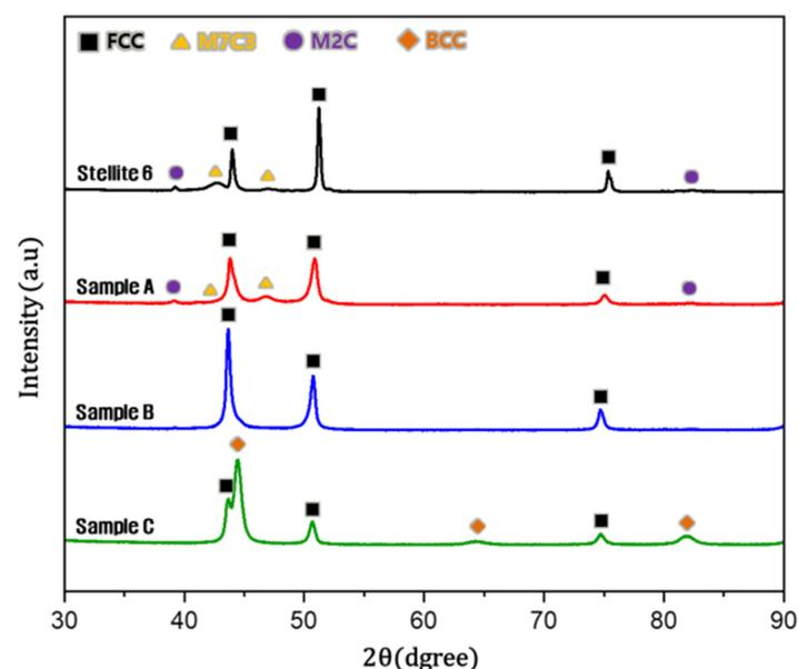
Figure 1. XRD phase analysis results of Stellite 6 according to the amount of Fe added.
