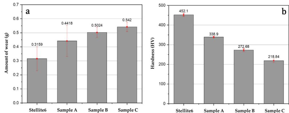
**Figure 5.** (a) Graph of changes in wear amount according to Fe content and (b) changes in hardness value according to Fe content.
