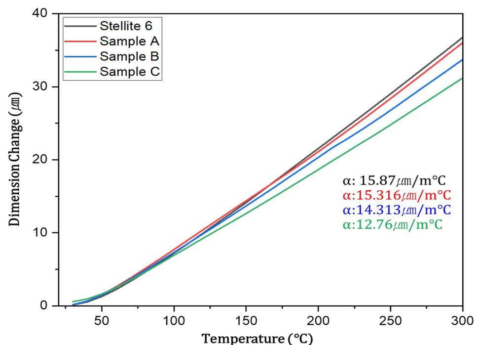
**Figure 8.** Results of the thermal mechanical analysis (TMA) for measuring and calculating the coefficient of thermal expansion (CTE).
