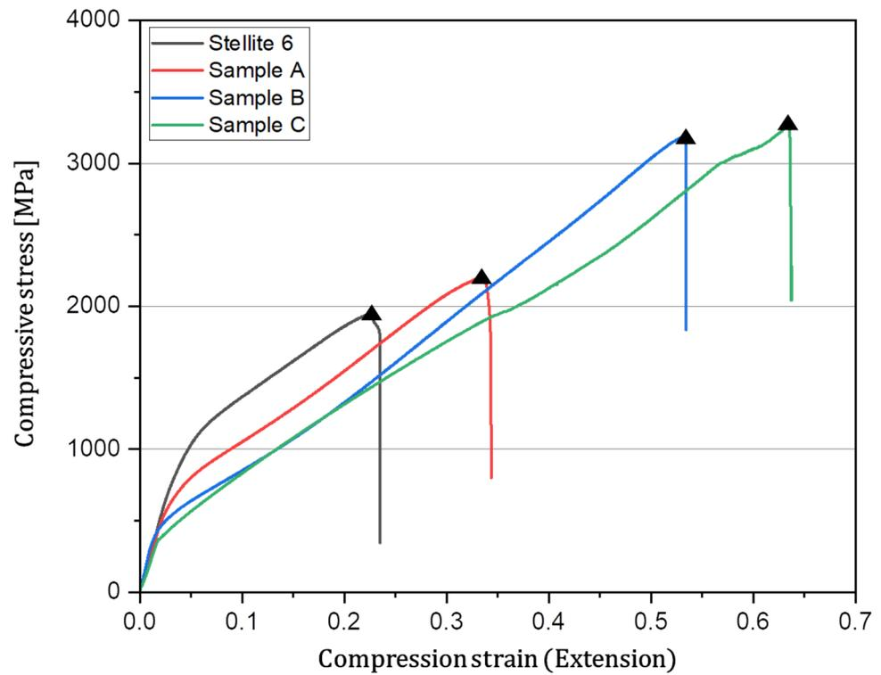
Figure 6. Graph depicting the stress–strain curves from the compression tests.
