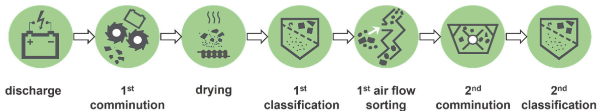
Figure 1. Recycling process to produce fragments of current collector foils.
