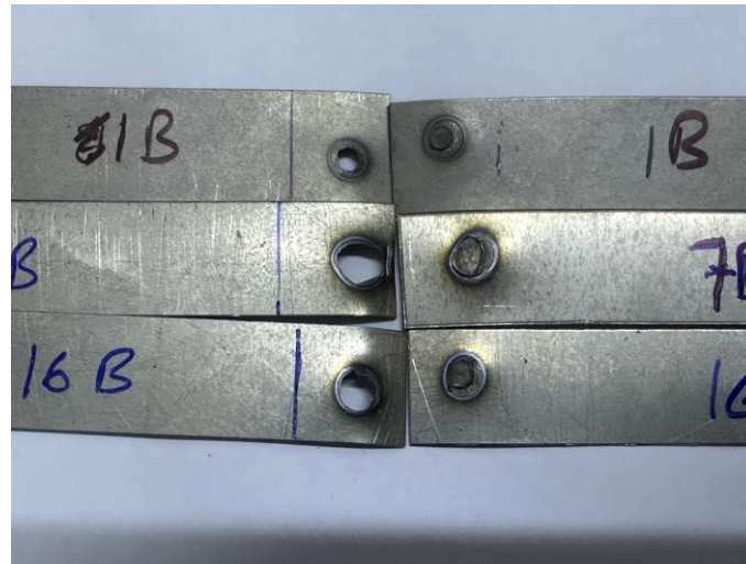
Figure 14. Pull-out nugget failure of case B.
