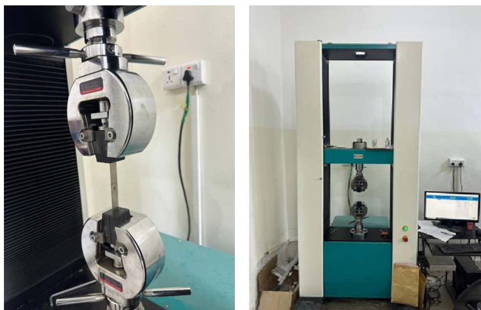
Figure 4. Tensile shear test of the RSW joints.
