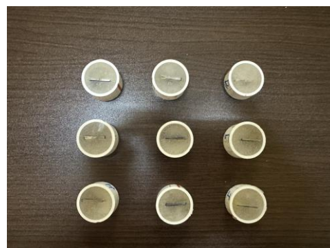
Figure 7. Mounted samples of microstructure and micro-hardness tests.
