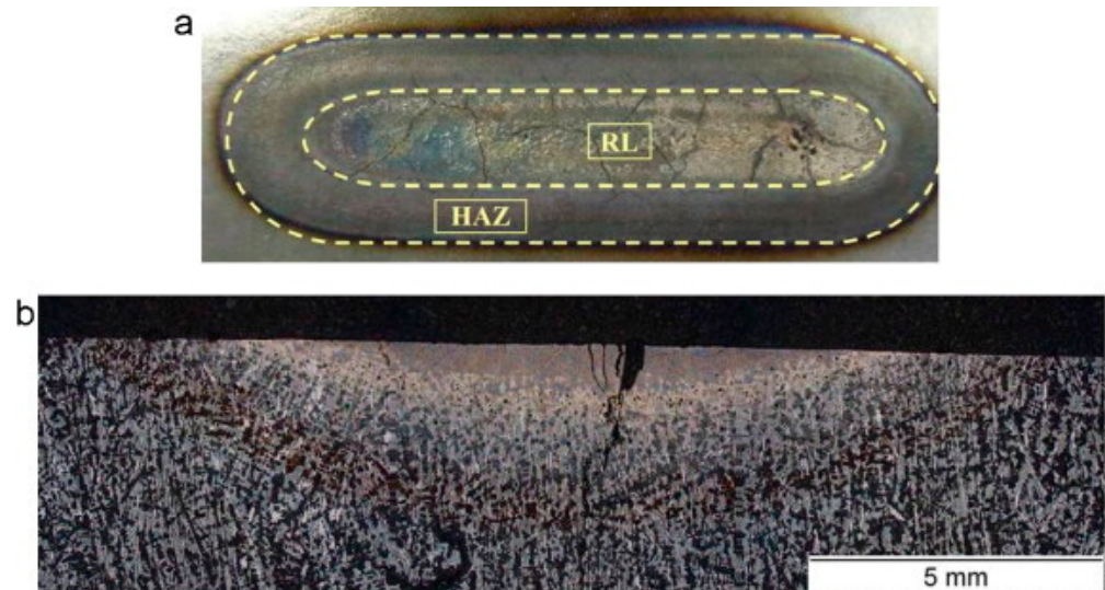
Figure 6. LSTH of cast iron: (a) top view of the hardening line; (b) cross-section of the sample (reproduced from Ref. [75], with permission from Elsevier, 2012).
