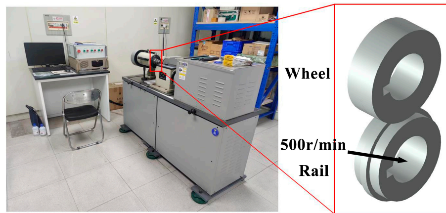
Figure 1. Schematic diagram of the contact mode between the test equipment and rail samples.
