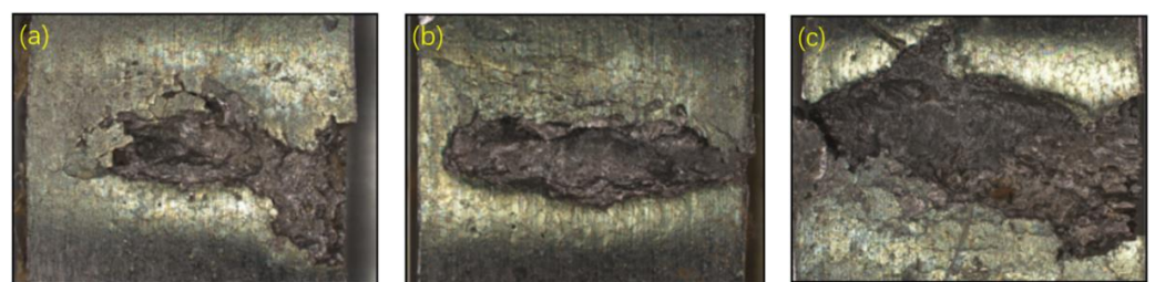
Figure 4. Peeling pit morphology under different stresses: (a) 1300 MPa, (b) 1400 MPa, and (c) 1500 MPa.
