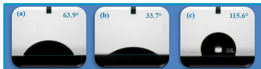
Figure 1. Contact angle of MAO film treated with (a) KH560, (b) BTSE, and (c) DTMS.
