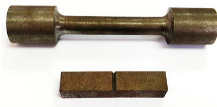
Figure 2. Ductile iron samples prepared for heat treatment.
