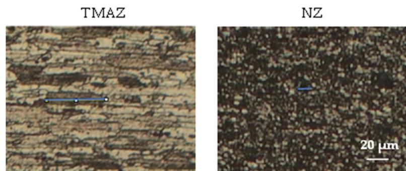
**Figure 13.** Grain size measurement using ImageJ for hot welding specimen.
