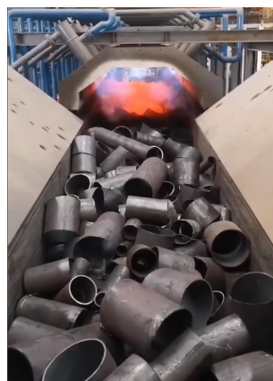
Figure 1. Horizontal preheating furnace.
