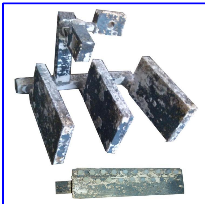
Figure 2. Large fabricated ceramic-reinforced TWIP steel matrix composite samples.
