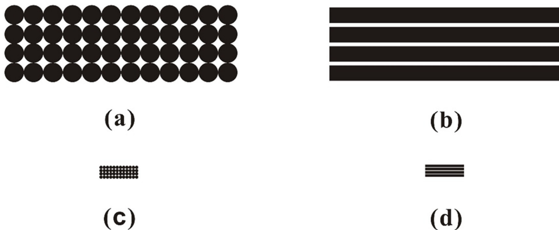
Figure 6. Different profiles of dislocation and the formation of dislocation patterns. (a,c) Point defect and PSB ladder on plane ( \bar{1}21 ); (b,d) line defect and PSB wall on plane (111).
