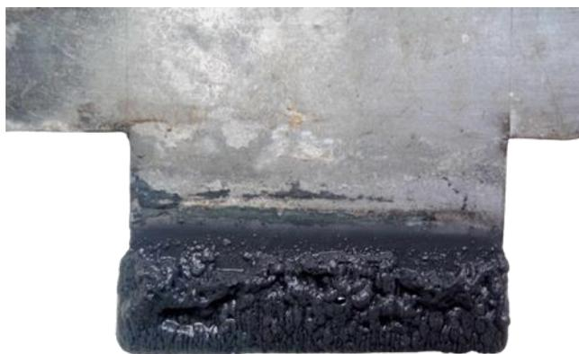
**Figure 7.** Zinc deposited on stainless steel cathode after electrodeposition of the pregnant solution obtained by alkaline leaching.
