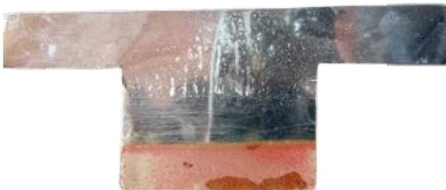
**Figure 6.** Stainless-steel cathode after electrodeposition with phosphoric acid pregnant solution.
