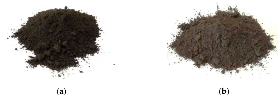
Figure 2. Manganese ore samples: (a) the Bogach deposit; (b) the Zhaksy deposit.
