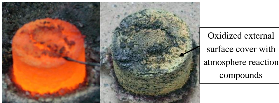
Figure 2. Reaction process and obtained SHS product without reactor.
