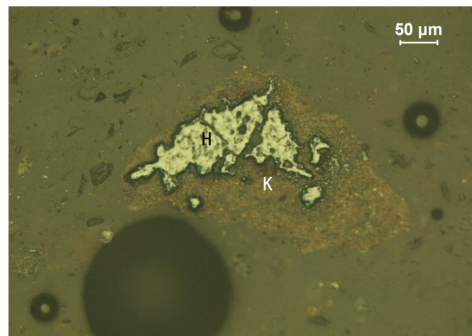
Figure 3. Granular hematite (H) filled in the particles of kaolinite (K) under reflected light.
