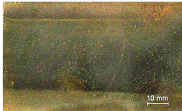
Figure 5. Burn-eroded surface of the sample made from steel EN X210Cr12 after WEDM.
