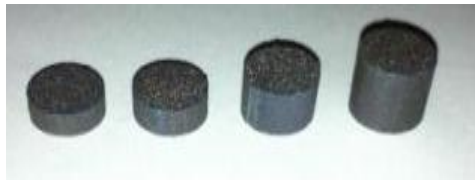
Figure 1. The final samples with the size of \phi 8 \text{ mm} \times 3 \text{ mm} , \phi 8 \text{ mm} \times 4 \text{ mm} , \phi 8 \text{ mm} \times 6 \text{ mm} and \phi 8 \text{ mm} \times 8 \text{ mm} .
