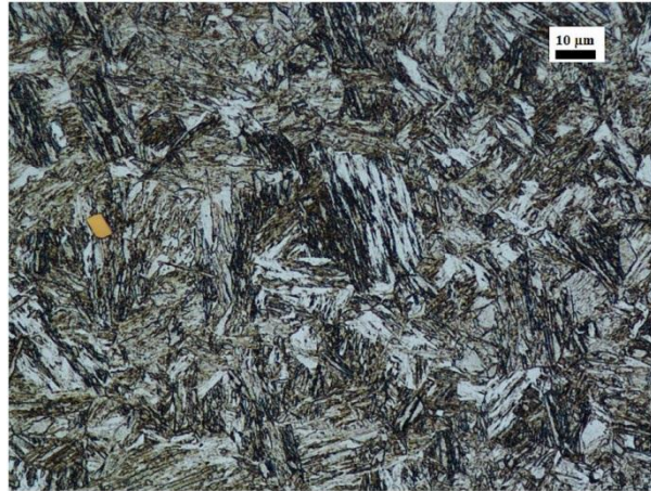
Figure 1. The microstructure of the investigated low-alloy boron steel with a high resistance to abrasive wear in the as-received state. Etched state, light microscope.
