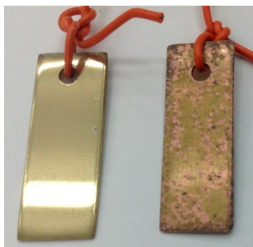
Figure 10. Samples (inhibited-left, uninhibited-right) for XPS-studies after 20 cycles in the salt fog chamber.
