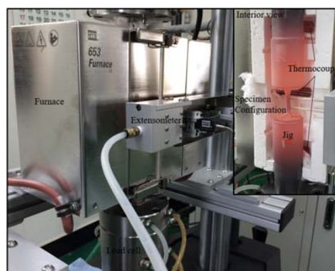
Figure 3. Apparatus and experimental setup of the LCF test.
