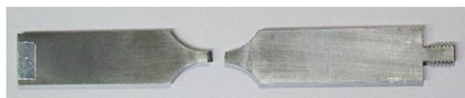
Figure 8. Specimen after the fatigue test.
