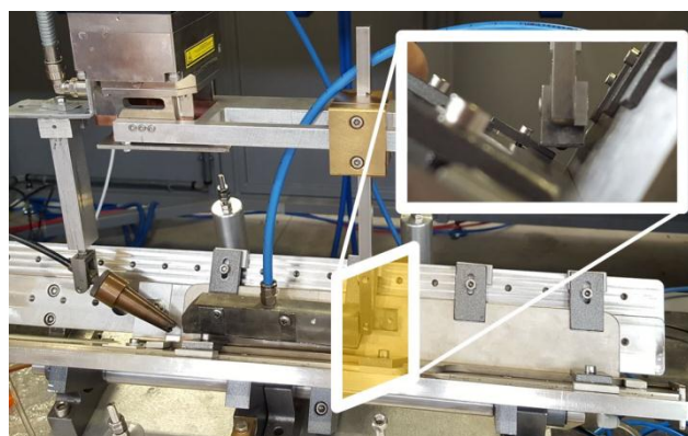
Figure 7. Positioning of the nozzle for plasma blow and the diffuser for inert shielding supply; back-side view in the inset.
